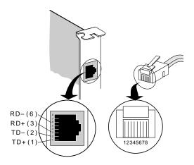
NOTE: When Category 5 UTP cable is used, the pin assignments are identical for 10Base-T and 100Base-TX.
