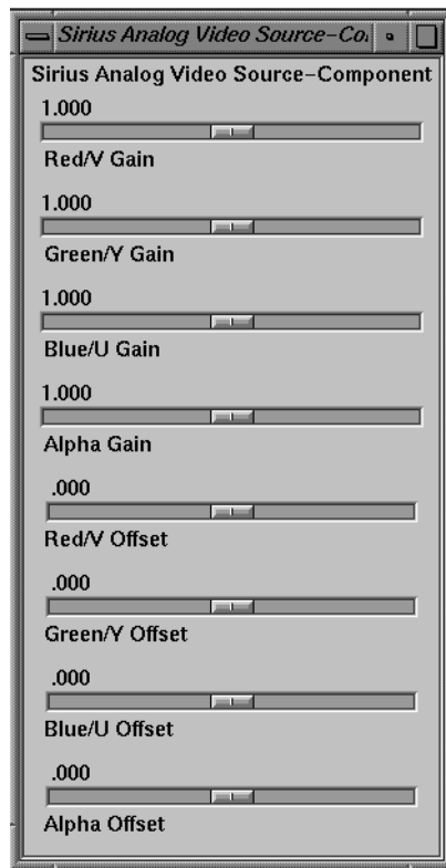
Figure C-12 Adjusting Gain and Offset for Component Video
