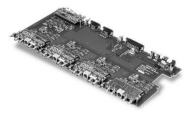
Each Quad Switch port can be configured with a different type of media card to perform media conversion between ports. For example, a cluster of four coax cards installed on ports 1 through 4, while a long-link fiber media card on port 5 could be used for the main ring connection to other Quad Switches separated by long distances.
